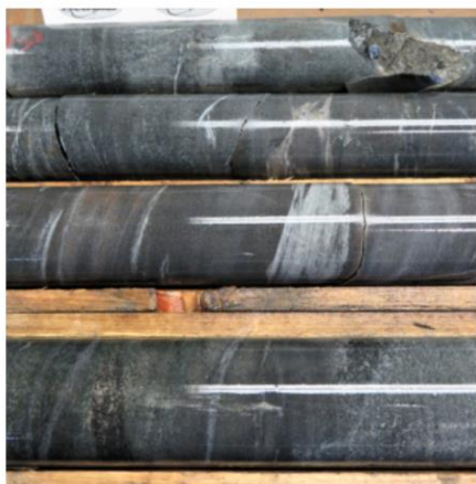
TESW-21-01: MINERALIZED ANDESITE FLOW, veins and sulfides stringers
