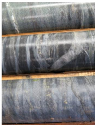
TESW-21-03: SILICIFICATION WITH BIOTITE - AMPHIBOLE disseminated chalcopyrite
