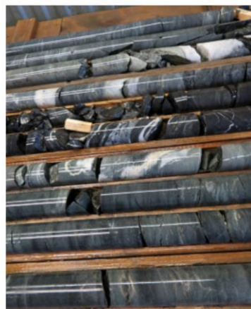
TESW-21-04: QUARTZ BRECCIA IN FAULT ZONE
